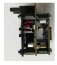
Train sensor module (without ultrasound transducer)
